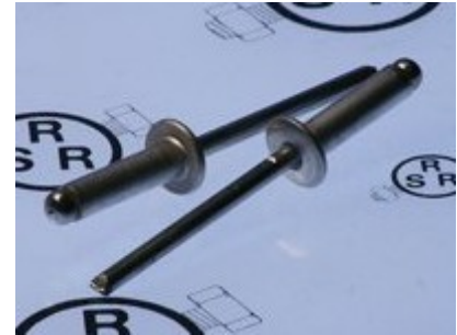
Rivet Body: Alu AlMg 3 Mandrel: A2 Stainless Steel
