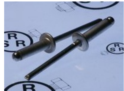
Rivet Body: AlMg 3 Mandrel: Steel Zinc Plated
